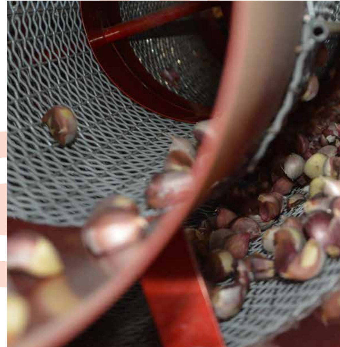
4 Great Diameter concentric drums cloves grader. The special grader with five separated exits, load the big boxes with regular cloves sizes at highest capacity. Cloves graded ready to be planted.
