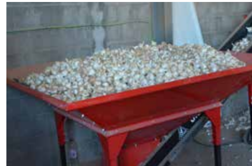
Big feeder hopper . Adjustable belt speed. Its 500 Kg capacity give autonomy for continuous garlic feeding to the cracker during enough time to be refilled and managing the sorted cloves boxes by only one person.
