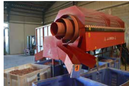
4 Great Diameter concentric drums cloves grader. The special grader with five separated exits, load the big boxes with regular cloves sizes at highest capacity. Cloves graded ready to be planted.
