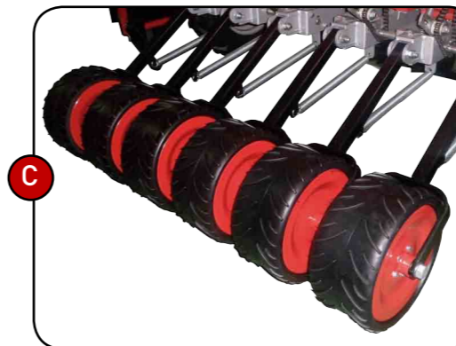
C. Compacting of bulbs by means of rear wheels (option).
